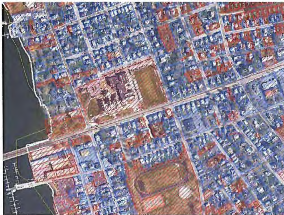
Figure 1. A portion of the MEP GIS coverage for Fairhaven. Blue areas are listed as sewered, red areas listed as on septic, and numbers show number of buildings on the parcel. Probably none of the properties shown in this area have septic systems.
