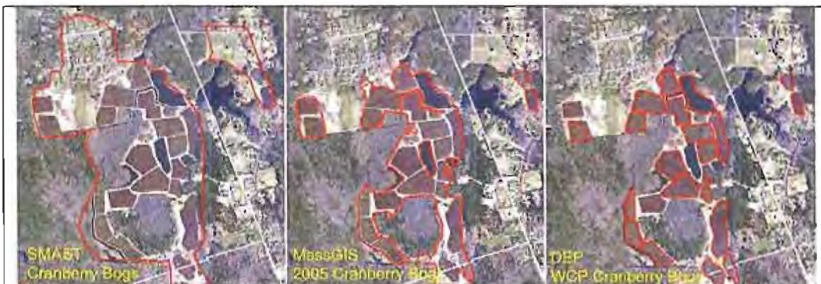
Figure 11. A comparison of MEP's newly created cranberry bog coverage in the Acushnet River watershed (left), versus MassGIS cranberry bog coverage in their 2005 land use data (middle), versus DEP wetlands conservancy program coverage. The DEP coverage is the most accurate estimate of production area, but needs to be manually updated based on the most recent aerial photographs.
