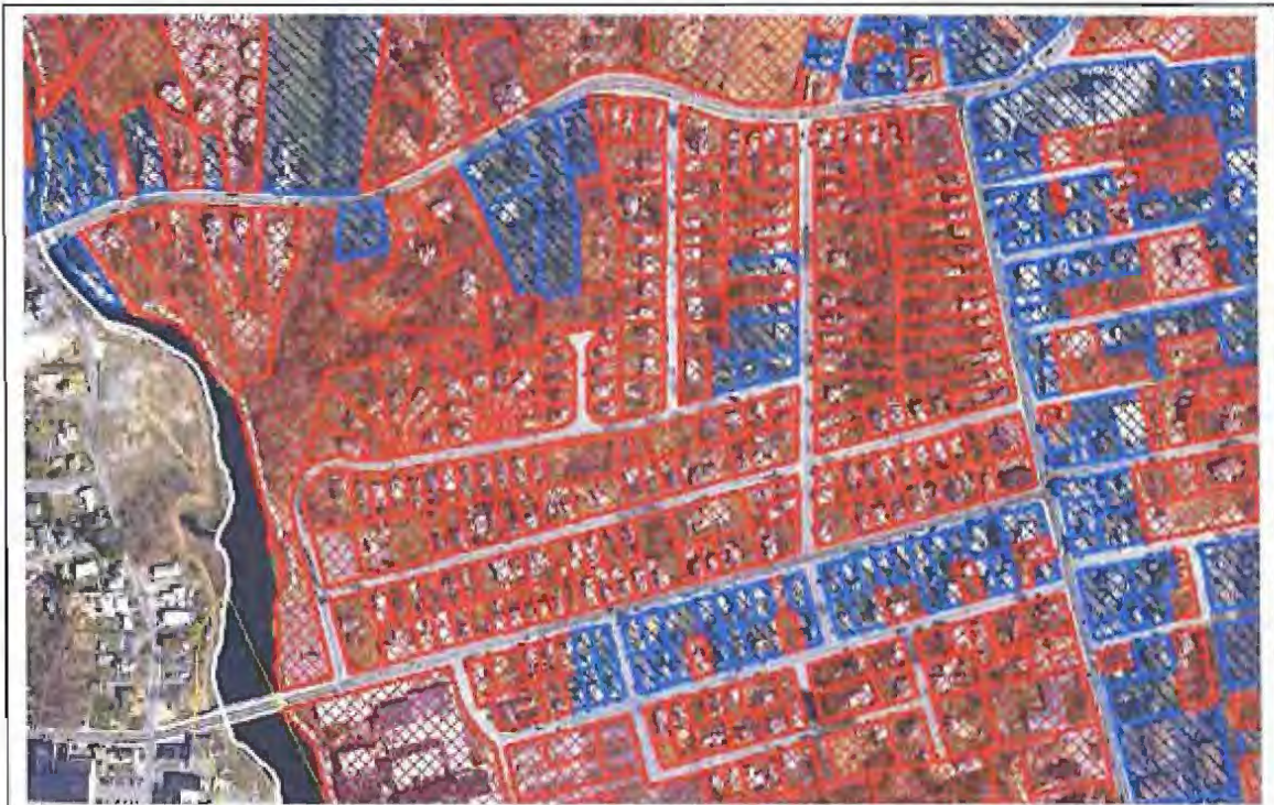
Figure 4. MEP data showing sewer service areas (blue crosshatch) and septic service areas (red crosshatch) in Acushnet, between Slocum St and Tarklin Hill Road. This areas was reported to us as sewer service and should be verified.
